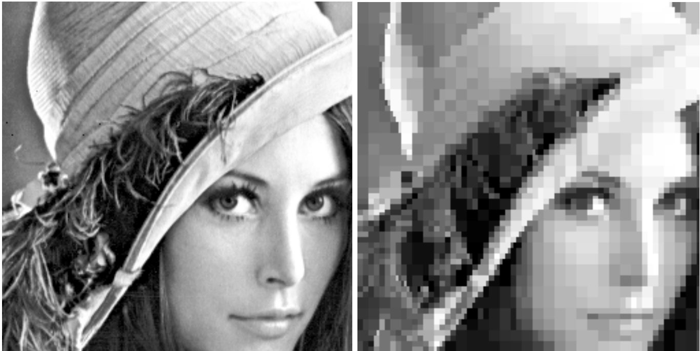
Fig. 21. A central part of the image ‘lenna’, original picture and restoration from the decomposition quantized with threshold 250.
