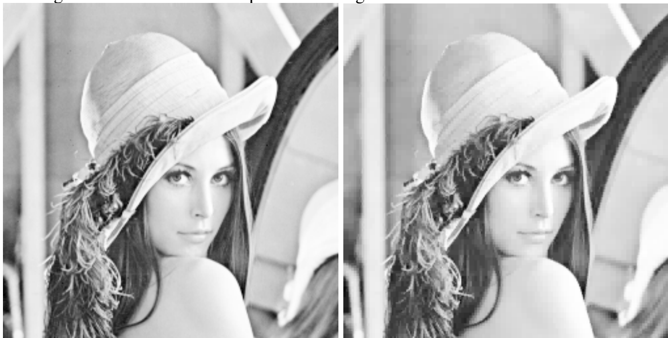
Fig. 14. Original and compressed image 'lenna', threshold 50, compression ratio 19:1, RMSE 6.60, L_1 error 4.25. Printed at scale 2:1 after the \gamma -correction with the factor 1.85.
